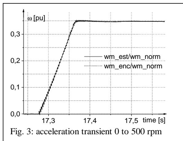
Fig. 3: acceleration transient 0 to 500 rpm
