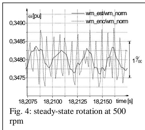
Fig. 4: steady-state rotation at 500 rpm
