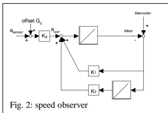
The other observer structure consists of one integrator which estimates the speed signal. This estimated speed signal is compared to the differentiated position information of the incremental encoder. This structure is less complex and therefore it is easier to place the eigenvalues in the Laplace-area. None of these observers needs special parameters of the machine. Therefore no parameter identification is necessary.
