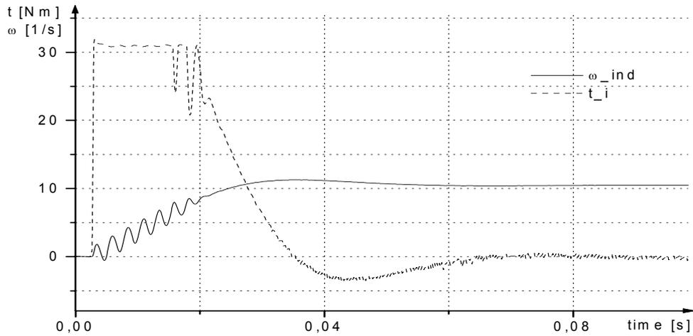
Fig. 4: Measured active damping of high frequency mechanical oscillation with the new torque control algorithm
