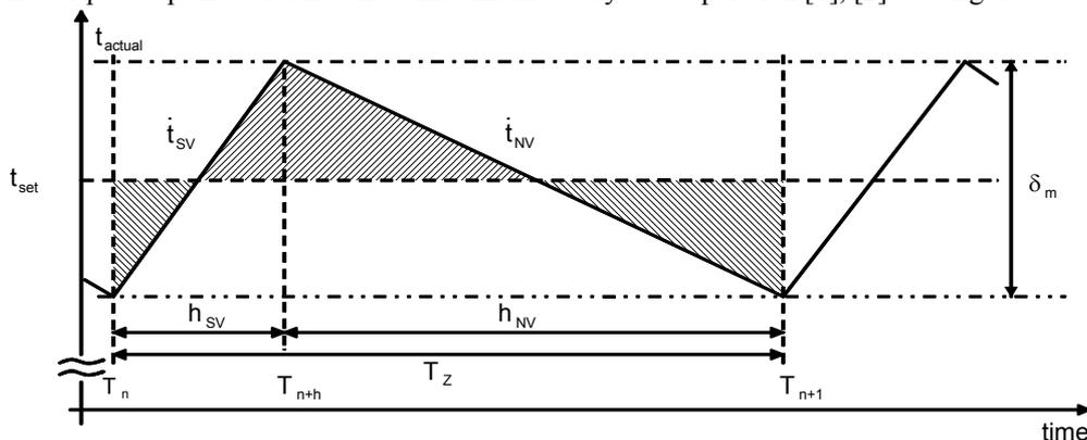
Fig. 1: Torque control cycle with DMTC
