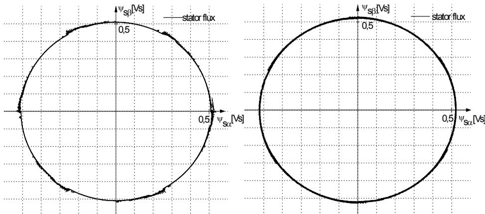
Fig. 3: Simulated stator flux of the induction machine at no load and 10 rpm (left) and 500 rpm (right)
