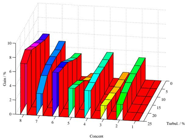
Figure 2: Energy Gain as a function of turbulence. Annual average windspeed  $7m/s$ , design tip speed ratio 6, profile Goe 758
