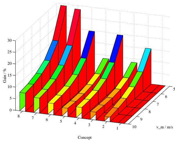
Figure 3: Energy Gain as a function of annual average windspeed. Turbulence 10%, design tip speed ratio 12, profile Goe 758
