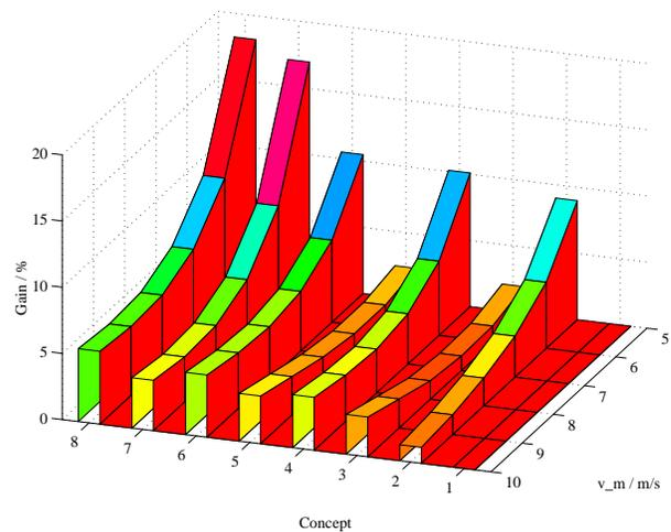
Figure 1: Energy Gain as a function of annual average windspeed. Turbulence 10%, design tip speed ratio 6, profile Goe 758
