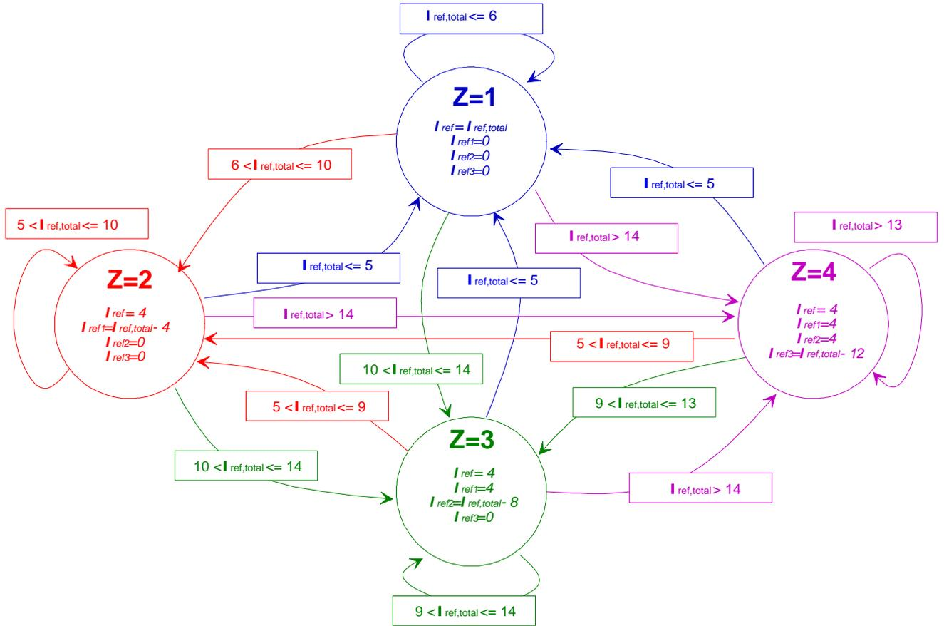
Fig. 3 State graph of the modified Load Distribution Control method
