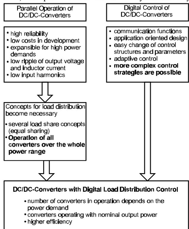
Fig. 1 Motivation for Digital Load Distribution Control
