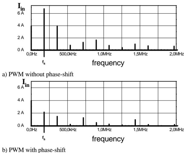
Fig. 4 Effect of the phase-shifted PWM on the input current spectrum
