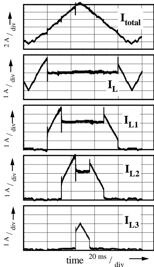
Fig. 8 Triangular current reference (LDC demonstration experiment)
