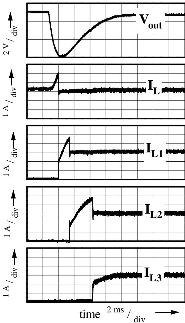
Fig. 7 Experimental measurement of sudden load variation from 3A to 12A
