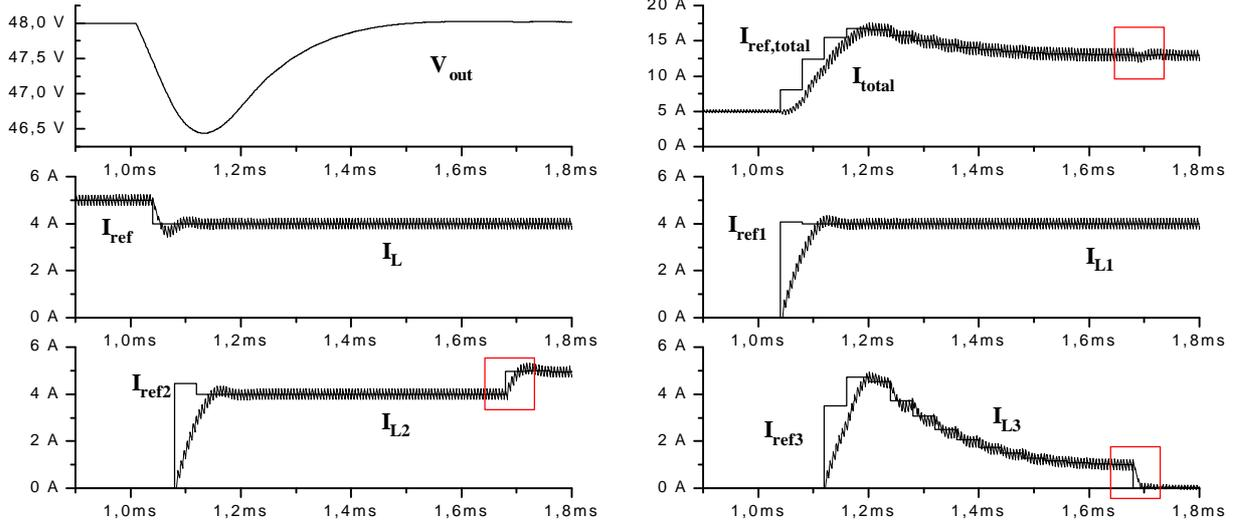
Fig. 6 Transient behaviour of the LDC after a sudden load variation at  $t = 1$  ms
